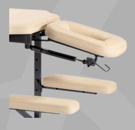
**Head section:** adjustable with a gas spring. **Height adjustment**: easy "1-click" system. **Armrests:** adjustable in height and distance, with optional side attachment in three positions.
